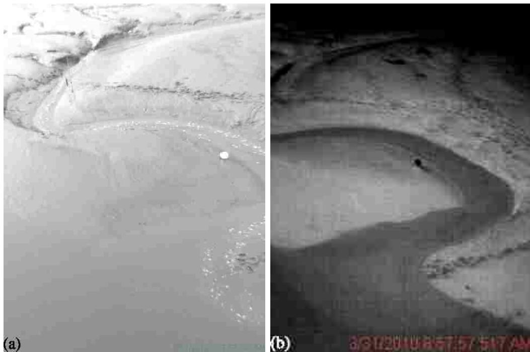
Figure 2.3 (a) Visual and (b) infrared imagery at Willapa Bay D Channel. Note how the contrast in the IR image is greater due to the large temperature differential between the exposed flats (lighter) and the water flowing out the channel (darker)
