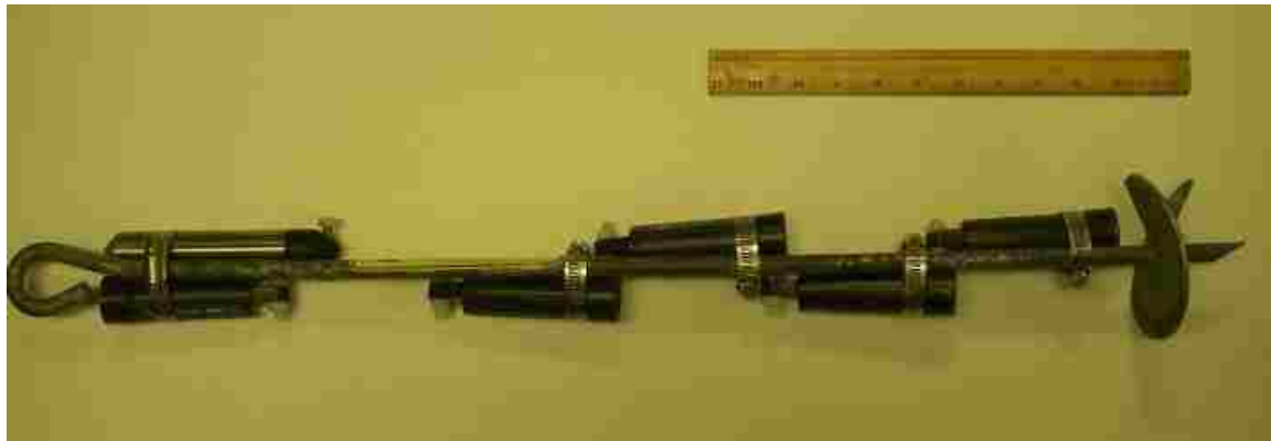
Figure 2.2 Sand anchors with affixed temperature loggers used in this study. A HOBO U20 water level logger is mounted at the top of the anchor and sits at the sediment surface with a co-located HOBO TempPro temperature logger. Four TempPro loggers are affixed at 10 cm intervals from 20 - 50 cm below the surface.
